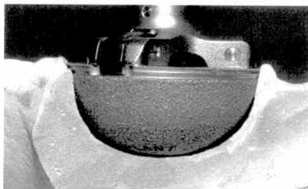
Fig. 1 Peripheral press-fit of the Durom ® cup may prevent contact with the prepared acetabular bone, particularly when preparation was performed with a hemispheric reamer of the same size. The sharp peripheral fins of the flared cup with a sector angle of 165° do not permit predictable, repeatable bone preparation, especially with recommended hemispheric reamers and hemispheric preparation.
